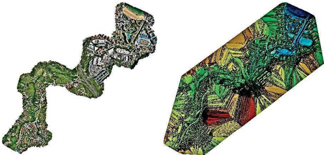
Figure 1: Orthomosaic and the corresponding sparse Digital Surface Model (DSM) before densification.
