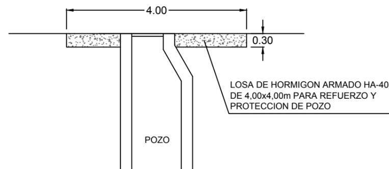
DETALLE LOSA DE REFURERZO POZO
